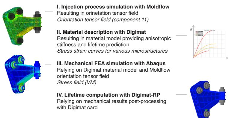
Figure 1: Integrative approach deployed by DSM to reach accurate lifetime prediction of SFRP parts
