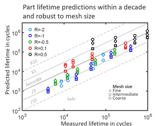
Figure 2: Correlation of predicted lifetime with test data covering different load ratios and multiple load amplitudes
