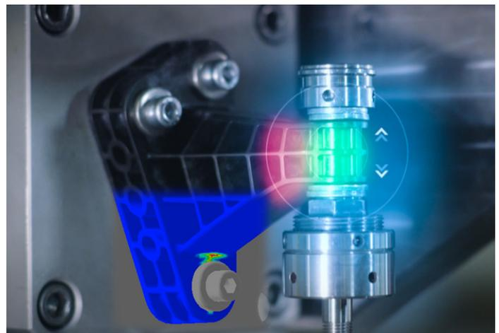
DSM load bracket, real testing and digital twin fatigue weak spot
