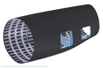
Fig. 1: Contoured fuselage barrel
