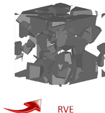
Generation of complex RVE based on geometric shape & size distribution
