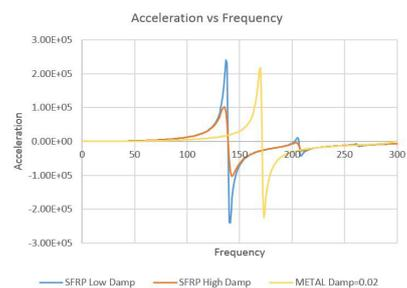
Figure 2: Highest and lowest damping curve identified through FEA at RVE level helps to provide an image of the response level range to be expected from the part
