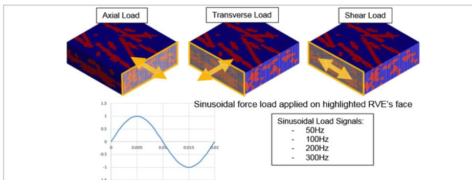
Figure 1: Material engineering through FEA at RVE level to identify the vibrational characteristics of the material
