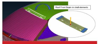
Prediction of the damping behavior of a roof front beam in NVH simulations
