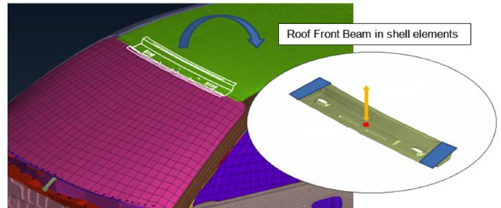
Prediction of the damping behavior of a roof front beam in NVH simulations
