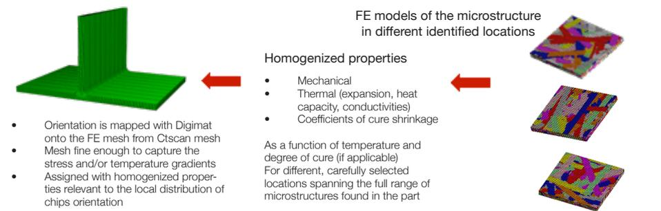
Figure 3: Methodology for the computation of the homogenized properties of DFC and transfer to the analysis mesh.
