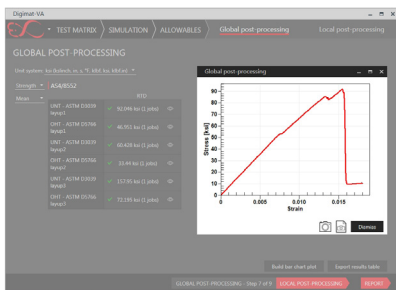
Figure 3: virtual allowable comparison with experiment for several laminates
