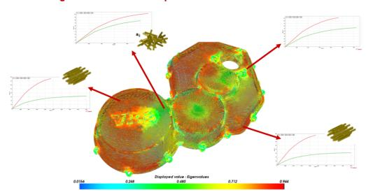
1. The local mechanical behavior is driven by the result of the manufacturing process: the fiber orientation distribution
