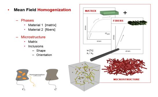
2. The multi-scale material modeling strategy is based on the Mori-Tanaka homogenization method applied on material models built on the matrix and reinforcement materials combined with the microstructure definition of the given reinforced plastic or composite.
