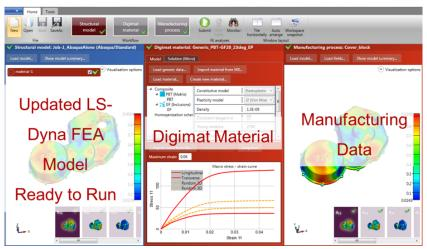
3. An efficient and quick tool dedicated to design engineer to set up LS-Dyna FE models with micromechanical material models and taking into account the manufacturing effect on the fiber orientation distribution for an accurate behavior prediction
