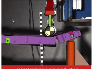
Impact test on a pre-production reinforced plastic front end carrier in the new Volvo XC90
